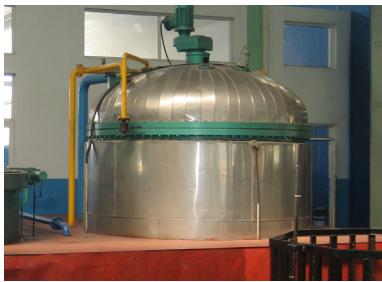
VPI Tank Vacuum Pressure Impregnation
